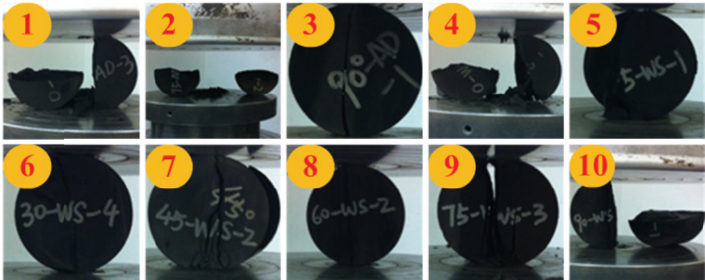
Fig. 9. Failure types in the Brazilian test Self-Elaboration
