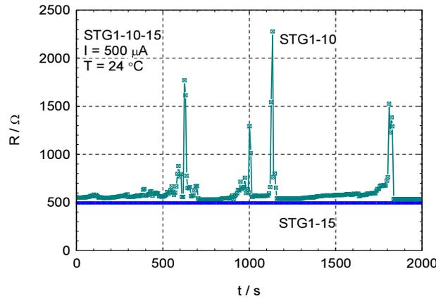
Fig. 2. Resistance vs. time for samples STG1-10 and STG1-15 for DC current  $I = 500 \mu\text{A}$  at a temperature of  $24^\circ\text{C}$ .
