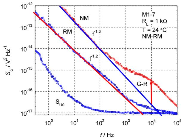
Fig. 8. Voltage noise spectral density vs. frequency for sample M1-7 for an applied voltage of 1.7 V,  $T = 24^\circ\text{C}$  and load resistance  $R_L = 1 \text{ k}\Omega$ , for RM (middle curve) and NM (upper curve). The lowest curve is the measuring set-up background noise spectral density  $S_{U0}$ .
