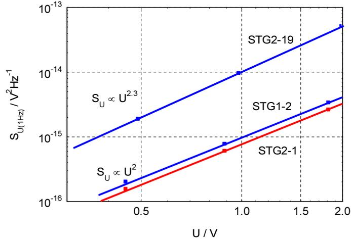
Fig. 9. The noise spectral density  $S_{U(1\text{Hz})}$  at  $f=1$  Hz vs. bias voltage  $U$  for samples STG1-2, STG2-1 and STG2-19 after subtraction of measuring set-up background noise measured at a temperature of  $T = 24^\circ\text{C}$ .
