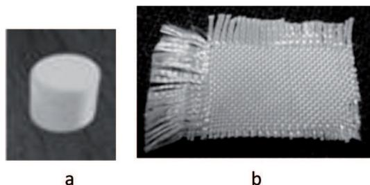
Fig. 2. Ceramic component (a) and aramid textile (b)
