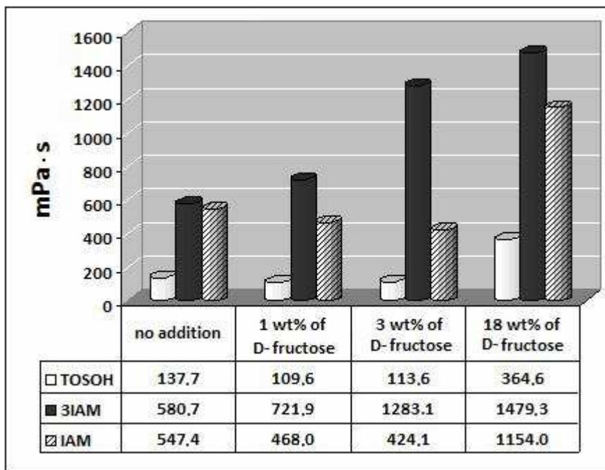
Fig. 1. Influence of D-fructose additive on viscosity of nanozirconia suspensions made of three different nano-ZrO<sub>2</sub> powders
