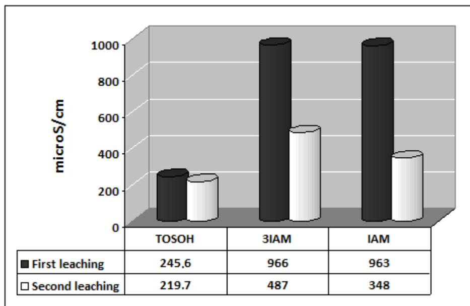
Fig. 2. Ionic conductivity of supernatants after first and second water leaching
