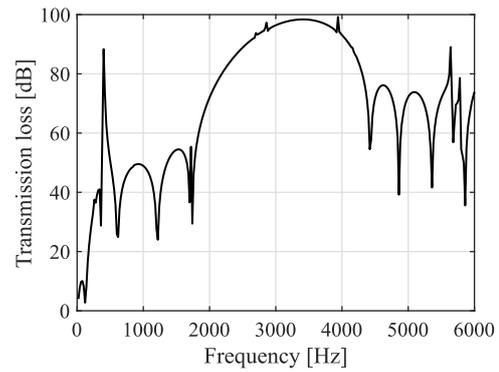
Fig. 6. TL through DPS with 2 rows of resonators.
