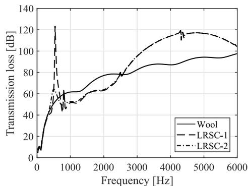
Fig. 5. TLs through DPSs with glass wool filling between two panels.
