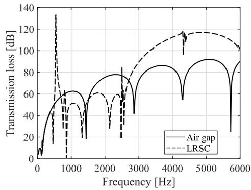
Fig. 4. TL through DPS with LRSC and that with air cavity.
