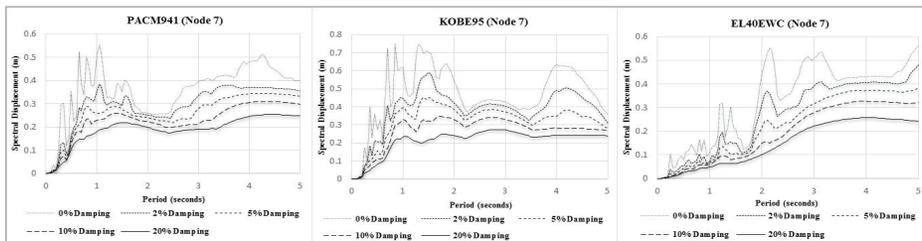
Fig. 5. Graph of spectral displacement versus time for three past earthquake records
