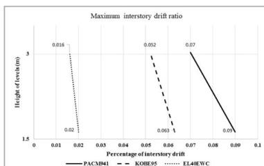
Fig. 7. Maximum interstory drift of the frame under three earthquake accelerograms
