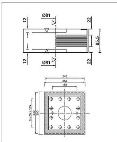
Fig. 2. Cross-section and side elevation of special base isolation unit [16]
