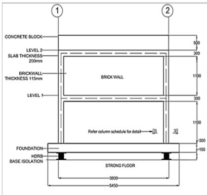
Fig. 1. Front view with dimensions of half-scale two-story RC frame with brick wall
