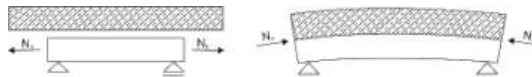
Fig. 3. Deformations of composite beams caused by temperature difference between wood girder and concrete (RC) beam
