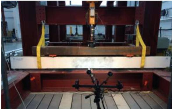
Fig. 3. Test setup with beam specimen
