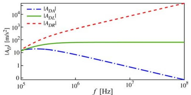
Fig. 2. Comparison of accelerations for  $|A_{DR}|$  radiation drift,  $|A_{DL}|$  viscous drift, and asymmetric drift  $|A_{DA}|$  in the ultrasonic standing wave field, for frequencies ranging from  $10^5$  to  $10^8 \text{ Hz}$ .
