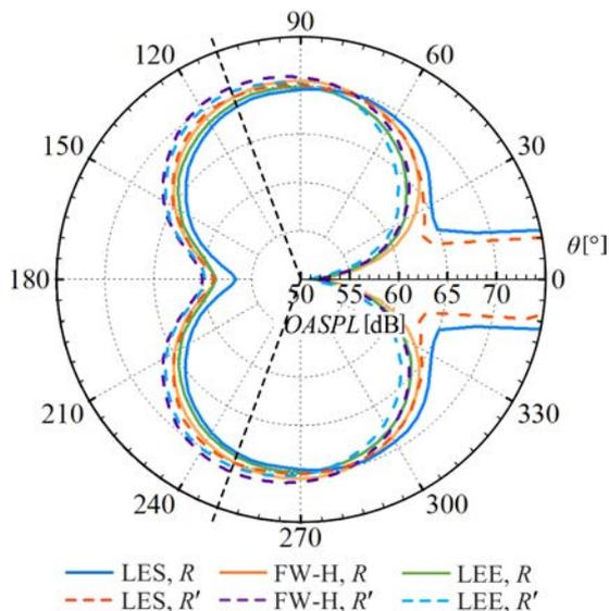
Fig. 10. Directivity of OASPL computed by LES, FW-H using HABC and the comparison with LEE. Solid lines denote the results at  $R = 20D_{\text{cyl}}$ ; dashed lines denote the results at  $R' = R(\sqrt{1 - M \sin^2 \theta'} - M \cos \theta')$  with  $R = 20D_{\text{cyl}}$ ,  $\theta' \in [-180^\circ, 180^\circ]$  (w.r.t. negative  $x$  axis).
