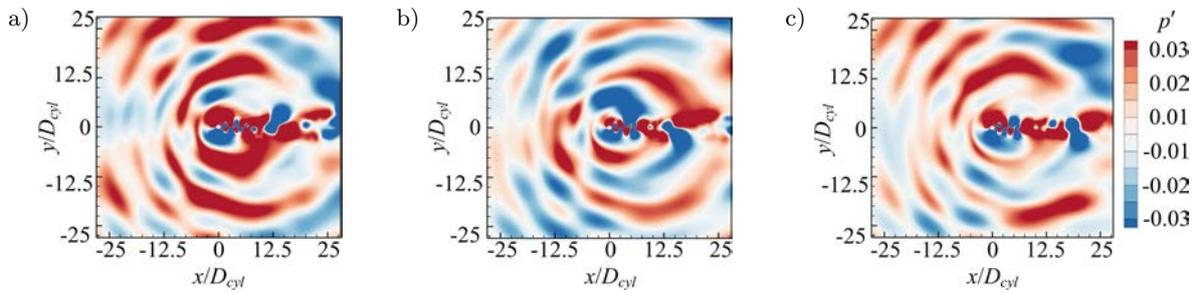
Fig. 3. Instantaneous contours of fluctuation pressure at the 262th vortex shedding cycle: a) baseline, b) Poinso BC, c) Far-field BC.
