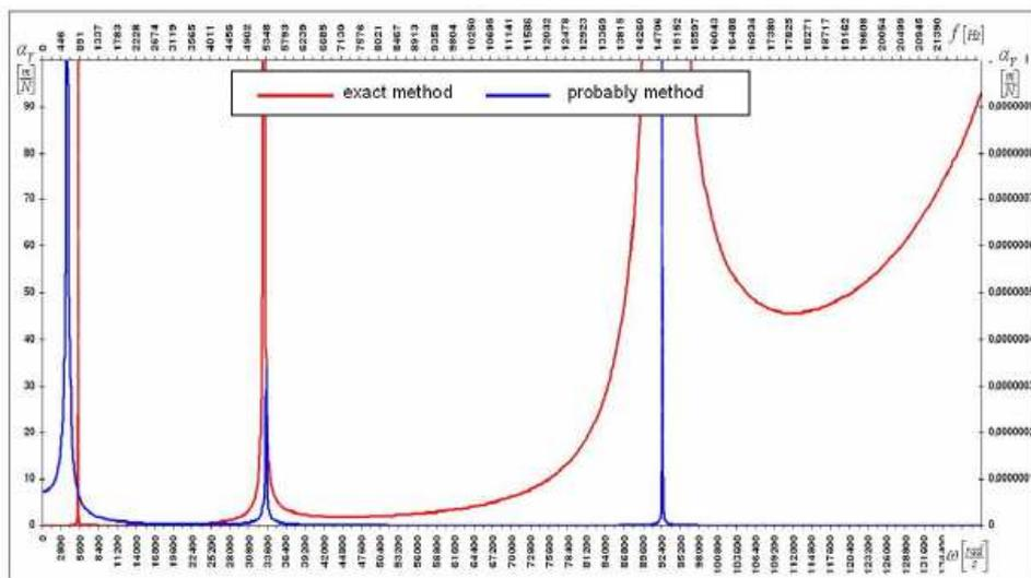
Fig. 2. The plot of absolute value of dynamical flexibility for the sum  $n=1, 2, 3$  mode vibration
