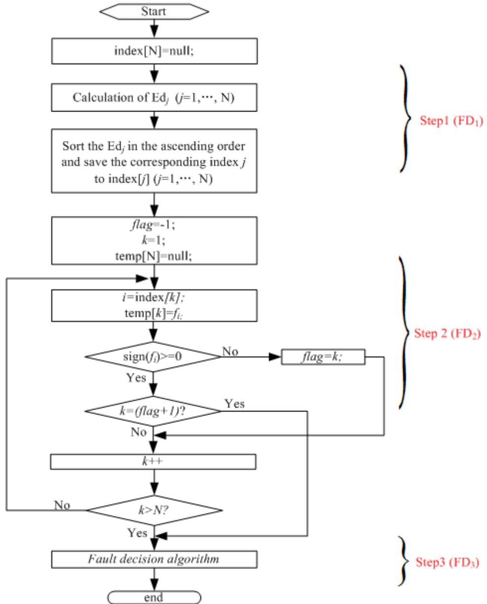
Fig. 5. Implementation flow chart of the proposed method.
