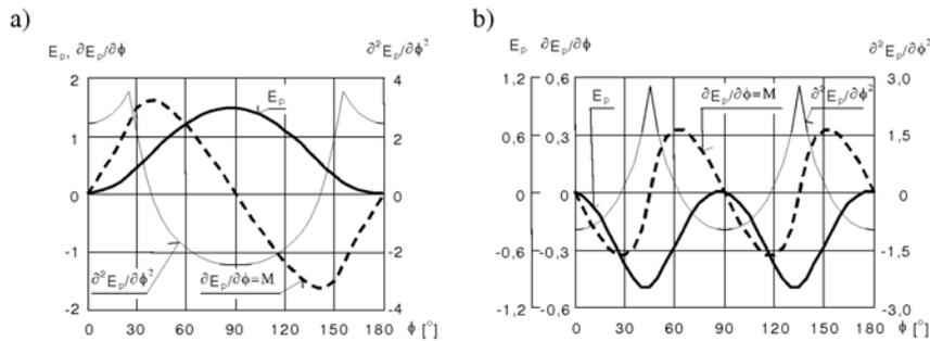
Fig. 6. The charts of potential energy of friction force moment  $E_p$  and its first and second derivative in the function of the angle of rotation of the load in the shape of: a) rectangle –  $a \times b = 0,4 \times 0,2$  m, b) square –  $a \times b = 0,4 \times 0,4$  m; initial load position on the conveyor  $y_0 = 0$ ,  $B = 0$  m,  $m = 5$  kg
