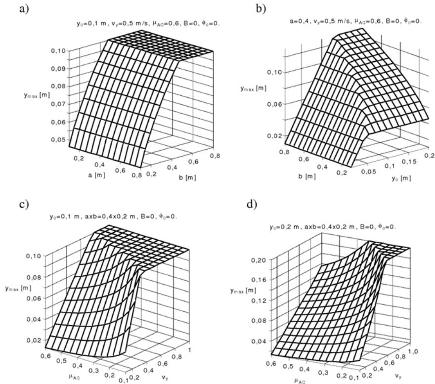
Fig. 4. Amplitude of oscillation of the load gravity centre determined in function of: a) load dimensions  $axb$ , b) initial position  $y_0$  of load on conveyor and load width  $b$ , c) friction coefficient  $\mu_{AC}$  and component of velocity  $v_y$  ( $y_0=0,1$  m), d) friction coefficient  $\mu_{AC}$  and component of velocity  $v_y$  ( $y_0=0,2$  m)
