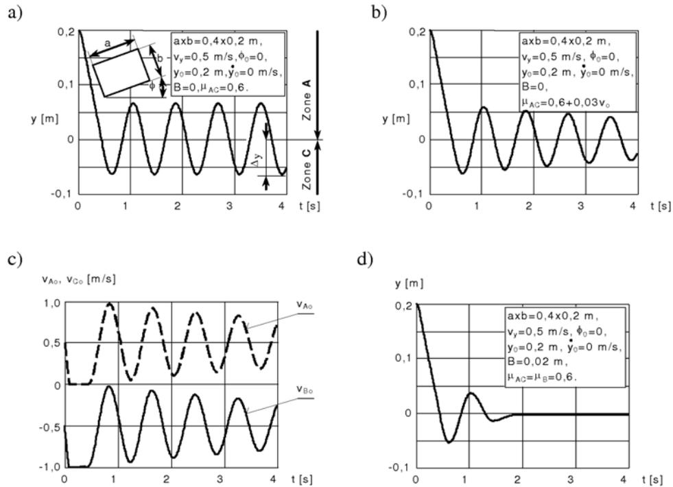
Fig. 3. The oscillations of the load motion obtained during simulation of positioning according to data: a) constant friction coefficient  $\mu_{AC} = 0.6 = \text{const}$  and  $B = 0$ , b) i) c) friction coefficient dependent on sliding velocity  $\mu_{AC} = 0.6 + 0.03v_0$  and  $B = 0$ , d) constant friction coefficient  $\mu_{AC} = 0.6 = \text{const}$  and  $B = 0.02$  m
