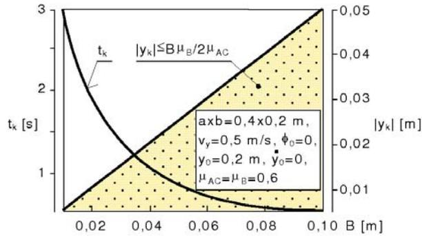
Fig. 5. An influence of width of zone B on the time  $t_k$  of the oscillation decay and precision of positioning (the position  $y_k$  of the load gravity centre after oscillation extinction)
