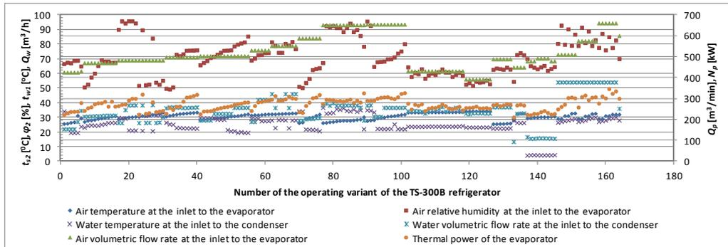
Fig. 1. Capacity of the evaporator and parameters of the air and water used in the statistical analysis
