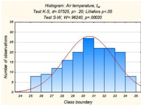
Fig. 2. Distribution of the air temperature at the inlet to the evaporator
