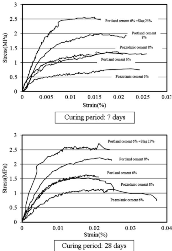
Fig. 4. Stress-strain curves for different types of binder
