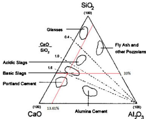
Fig. 3. Ternary diagram of binders (Hassani et al., 1998)
