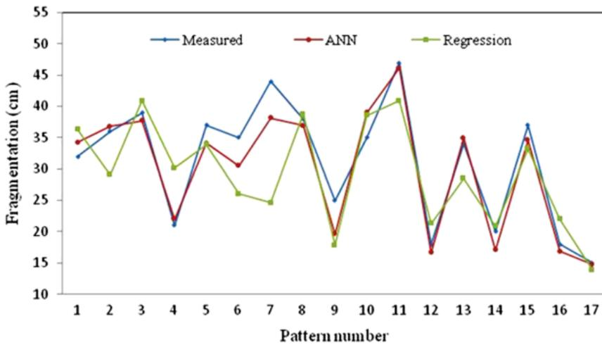
Fig. 6. Comparison of measured and predicted fragmentation
