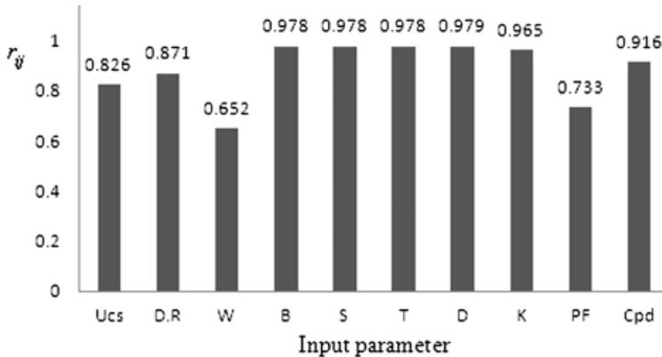
Fig. 7. The effect of input parameters on fragmentation
