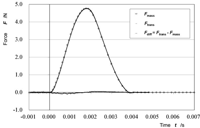
Fig. 4. Force calculated from output signal of the force transducer and its static calibration results  $F_{trans}$ , force acting on the mass  $F_{mass} (=Ma)$ , and their difference  $F_{diff} = F_{trans} - F_{mass}$ . Damper-A was used.
