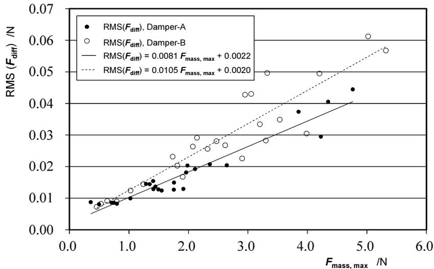
Fig. 6. Root mean square (RMS) values of the errors of the force  $F_{\text{diff}} = F_{\text{trans}} - F_{\text{mass}}$  measured with Damper-A and Damper-B.
