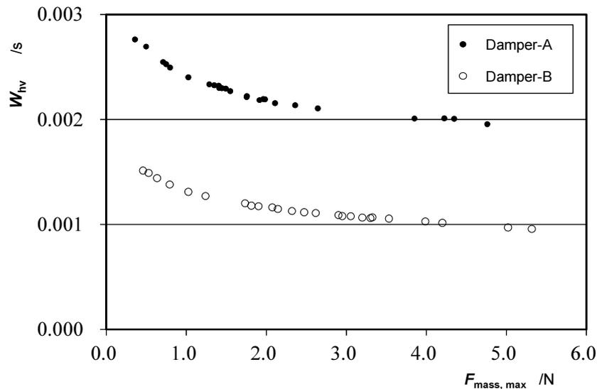
Fig. 5. The full width at half maximum  $W_{FWHM}$  against the maximum impact force  $F_{mass, max}$  as measured with Damper-A and Damper-B.
