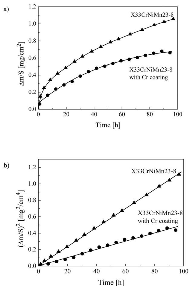
Fig. 1. Comparison of the oxidation kinetics of coated and uncoated X33CrNiMn23-8 steel at  $T = 1173$  K in air ( $\Delta m/S$  – weight changes of the oxidized sample per unit surface area): a) linear plot of coordinates, b) parabolic plot of coordinates
