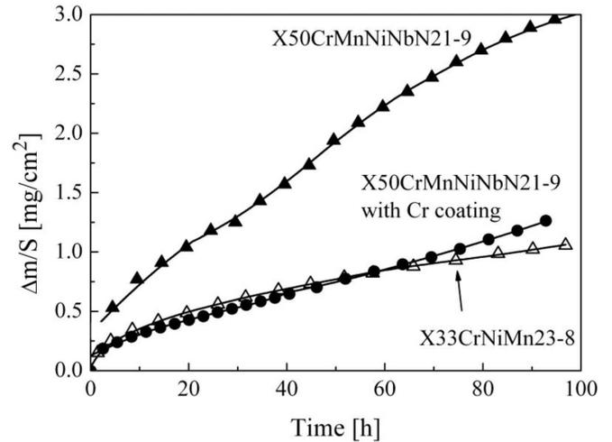
Fig. 3. The comparison of oxidation rate of the uncoated and coated X50CrMnNiNbN21-9 steel on the background of the analogous results obtained during oxidation of the uncoated X33CrNiMn23-8 steel
