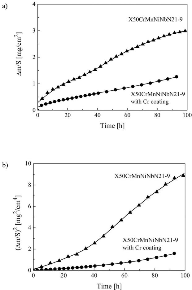
Fig. 2. Comparison of the oxidation kinetics of coated and uncoated X50CrMnNiNbN21-9 steel at  $T = 1173$  K in air ( $\Delta m/S$  – weight changes of the oxidized sample per unit surface area): a) linear plot of coordinates, b) parabolic plot of coordinates
