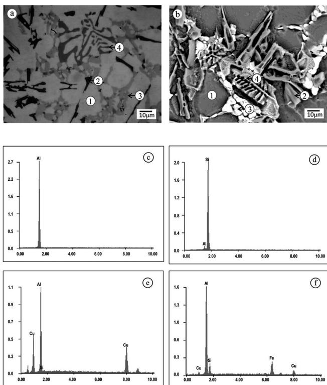
Fig. 2. (a) Optical micrograph and (b) SEM-BEI show the microstructure of the as-cast (AC) specimen. (c-f) Corresponding EDS spectra of  $\alpha$ -Al (marked '1'), Si (marked '2'), Al<sub>2</sub>Cu (marked '3') and Al<sub>5</sub>FeSi (marked '4'), respectively
