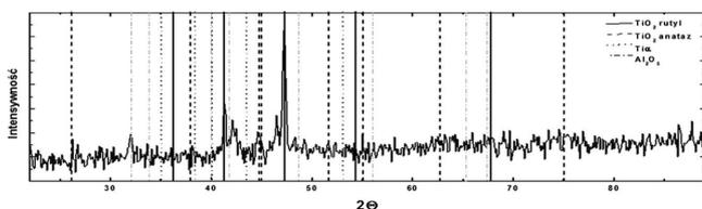
Fig. 3. X-ray pattern obtained for the oxidized surface of Ti-1Al-1Mn alloy
