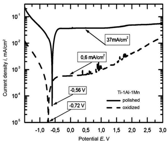
Fig. 6. Potentiokinetic polarization curves of Ti-1Al-1Mn alloy. Experimental conditions: artificial saliva solution, potential scan rate  $10 \text{ mV s}^{-1}$ , temperature  $37^\circ\text{C}$
