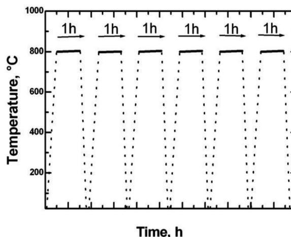
Fig. 1. Scheme of cyclic thermal oxidation of Ti-1Al-1Mn alloy
