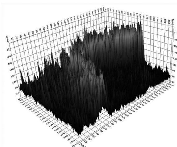
Fig. 4. The image of the Ti-1Al-1Mn alloy surface after 6 hours of oxidation (a), the surface topography of the selected area (b)
