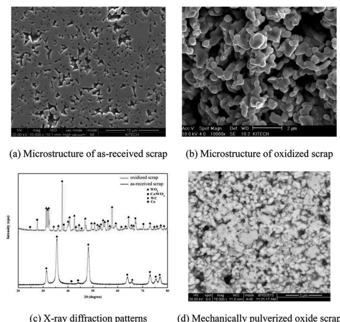
Fig. 2. Characteristic features of as-received scrap, oxidized scrap, and pulverized oxide scrap
