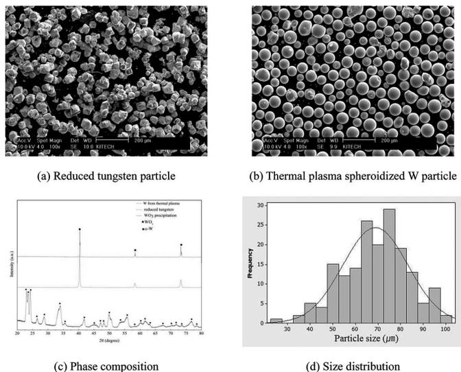
(a) Reduced tungsten particle (b) Thermal plasma spheroidized W particle
