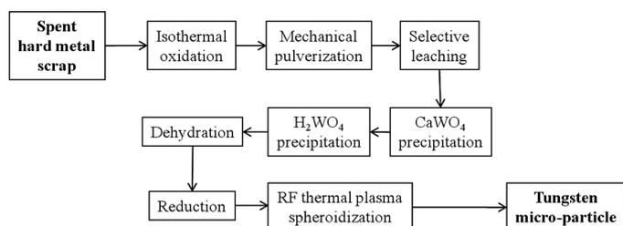
Fig. 1. Process flow of the combined recycling process
