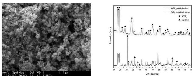
(a)  $WO_3$  powder from hydrometallurgy (b) Phase evolution during  $WO_3$  preparation
