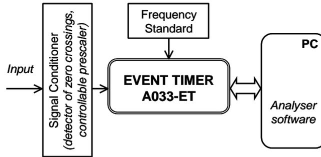
Fig. 2. Simplified block diagram of Jitter Analyzer.
