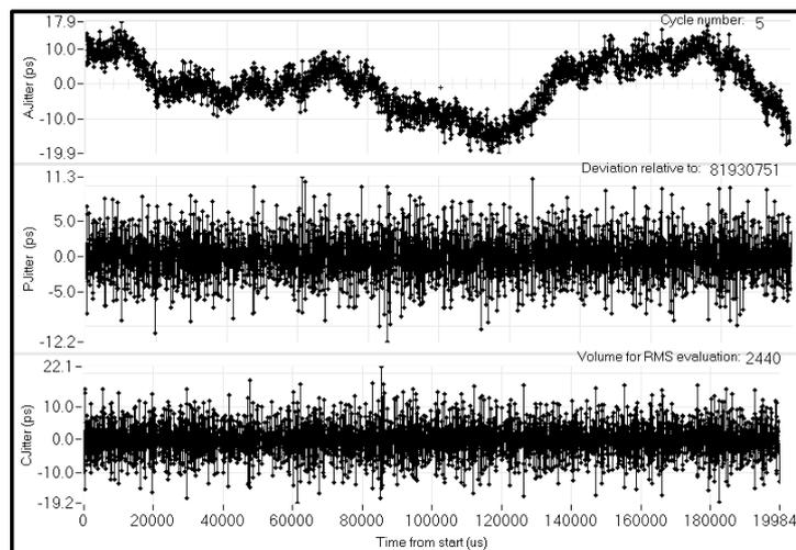
Fig. 3. Crystal clock generator jitter vs. time (1000 clock pulses).
