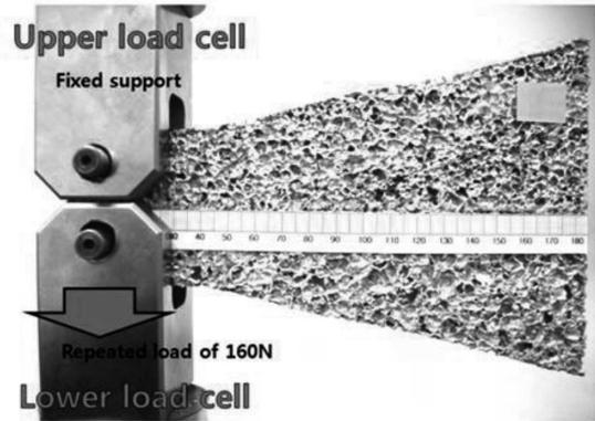
Fig. 3. Experimental setup at fatigue experiment
