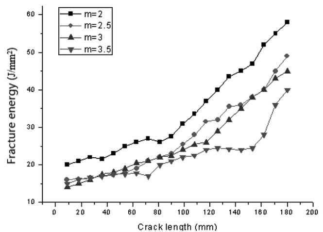
Fig. 7. Graph of fracture energy due to crack length (fatigue experiment)
