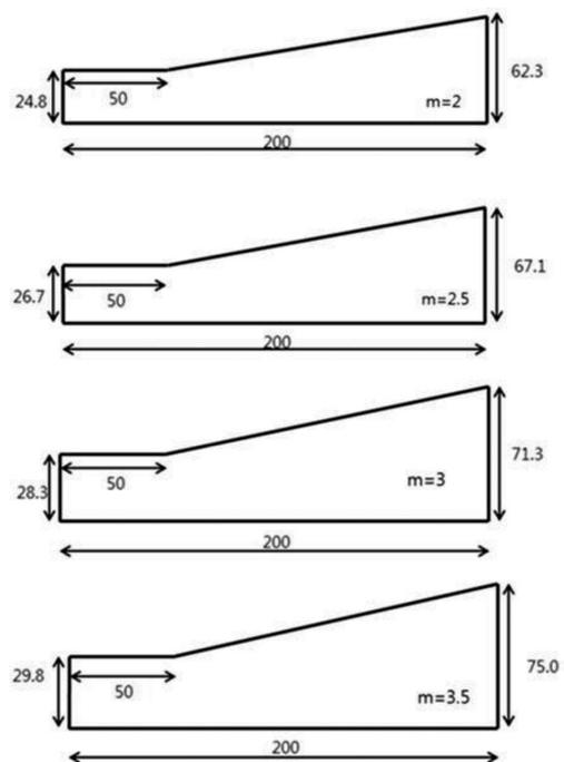
Fig. 5. Dimension of each specimen
