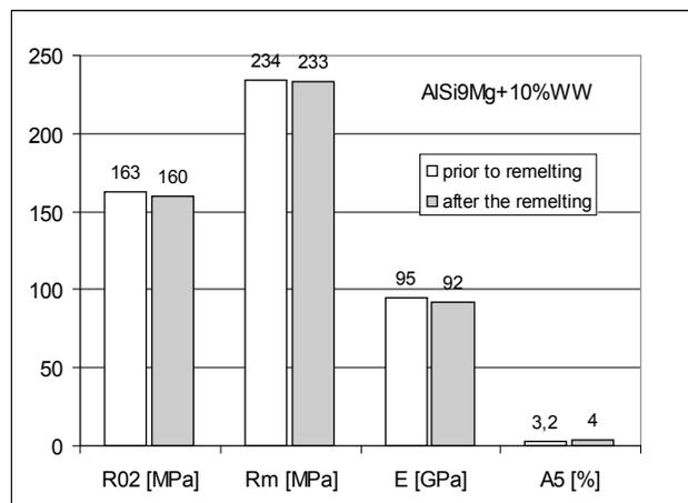
Fig. 5. Mechanical properties of AlSi9Mg alloy/10% CF prior to and after the remelting
