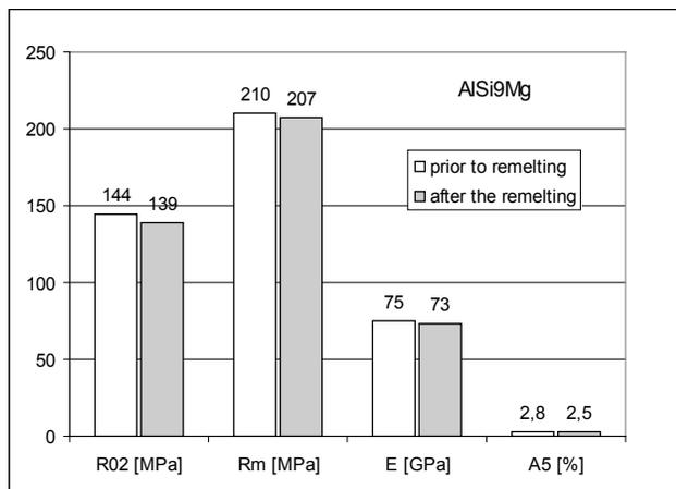
Fig. 4. Mechanical properties of AlSi9Mg alloy prior to and after the remelting
