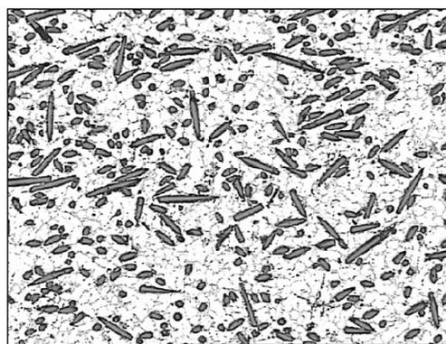
Fig. 2. Microstructure of the AlSi9Mg/10% CF composite, magn. 100 $\times$
