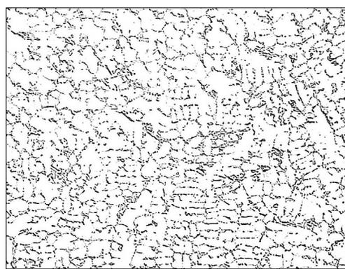
Fig. 1. Microstructure of the remelted AlSi9Mg alloy, magn. 100 $\times$
