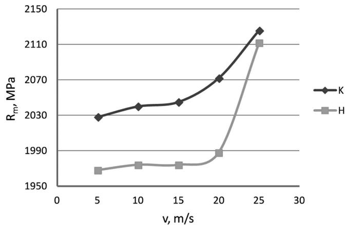
Fig. 4. The changing of ultimate tensile strength  $R_m$  for  $\varphi 1.7$  mm final wires drawn in conventional (K) and hydrodynamic (H) dies in drawing speed function
