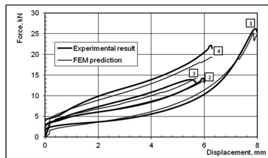
Fig. 1. Force-displacement curves obtained from compression tests 1-4 and their prediction calculated using flow stress given by equation (1)
