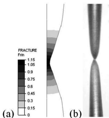
Fig. 3. Tensile test at 300°C with tool velocity equal to 1 mm/s: (a) ductility function; (b) fractured specimen.
