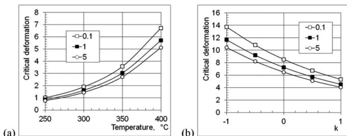
Fig. 4. Critical deformation for different temperatures (a), stress triaxialities (b) and strain rates
