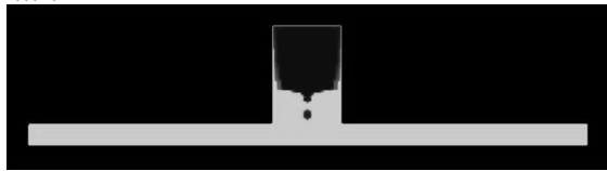
Fig. 8. Example of shrinkage defects obtained from solidification simulation of a steel casting aimed at finding efficiency of cylindrical feeders ( h/D=1.5 ); the feeder's dimensions determined from the modulus condition permitted to avoid shrinkage in the casting in this case
