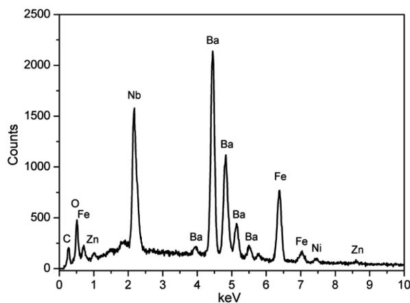
Fig. 3. EDS analysis for the BFN-NZF composite
