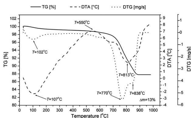
Fig. 1. DTA, TG and DTG curves of the BFN-NZF composite
