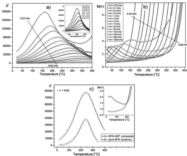
Fig. 5. Temperature dependencies of electric permittivity  $\varepsilon$  (a) and of the tangent of dielectric losses  $\tan\delta$  (b) of the BFN-NZF composite (heating). Inset Fig. 5a  $\varepsilon(T)$  for pure BFN ceramics. Comparison plots of the  $\varepsilon(T)$  and  $\tan\delta(T)$  for BFN-NZF composite and pure BFN ceramics, for  $\nu = 1$  kHz (c)
