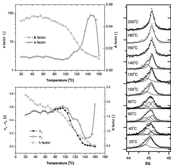
Fig. 6. Parameters obtained by fitting Preisach distributions using DAT function (left); XRD patterns of (200) reflection together with fitting results, circles – experimental data, lines – fitting results (right)
