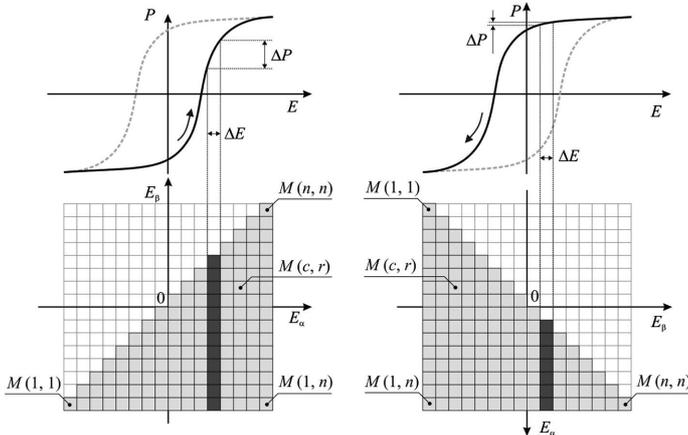
Fig. 2. Splitting the hysteresis loop into two curves, for increasing values of the electric field  $P(E)_{inc}$  (left), and decreasing field curve for  $P(E)_{dec}$  (right). Relation between  $\Delta P_{inc}$  (left) and  $\Delta P_{dec}$  (right) and Preisach distribution matrix element  $M(c, r)$
