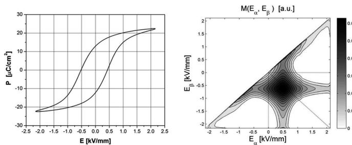
Fig. 3. Electric polarization ( $P$ ) versus electric field ( $E$ ) hysteresis loop for 0.775PMN-0.225PT sample at 70°C (left), and obtained Preisach matrix represented by density map (right)
