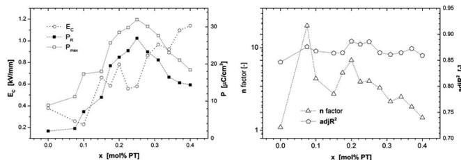
Fig. 7. Dependencies of parameters from hysteresis loops (left), and obtained by nonlinear fitting hysteresis loops function
