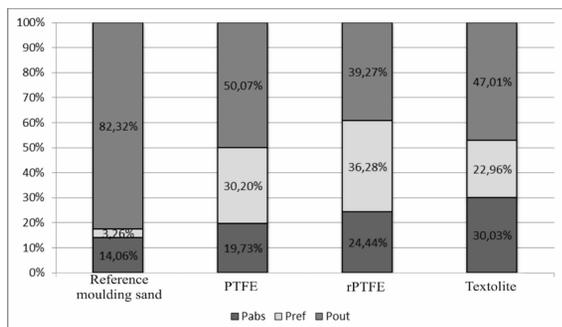
Fig. 3. Collective comparison of power indices  $P_{abs}$ ,  $P_{ref}$  and  $P_{out}$  measured for multimaterial systems with diaphragms made of the materials mentioned in Table 2
