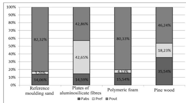
Fig. 2. Collective comparison of power indices  $P_{\text{abs}}$ ,  $P_{\text{ref}}$  and  $P_{\text{out}}$  measured for multimaterial systems with diaphragms made of the materials mentioned in Table 1
