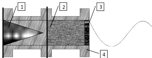
Fig. 1. Measuring assembly of the stand of microwave slot line: 1 – waveguide attenuator of microwaves; 2 – reference moulding sand; 3 – diaphragm plate; 4 – chamber filled with the examined multimaterial system
