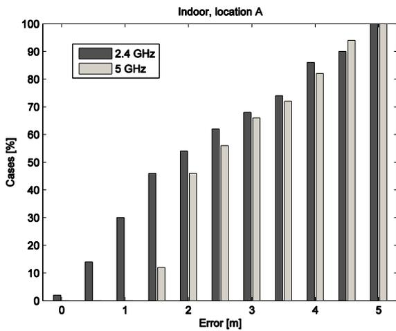
Fig. 5. Cumulative histogram of positioning error for location A.
