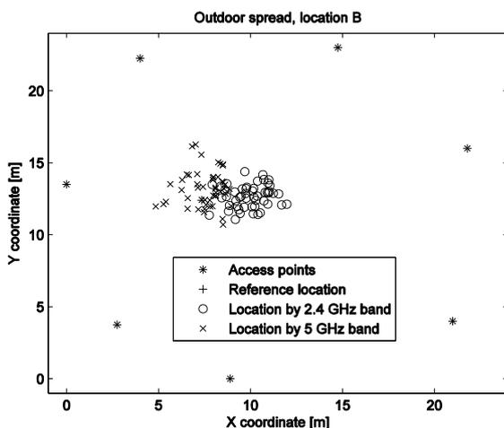
Fig.17. Positioning spread at location B (7.35, 12.4).
