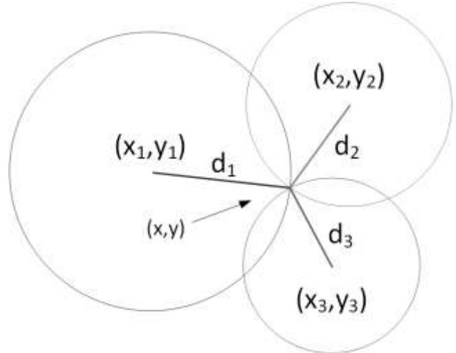
Fig. 2. 2D trilateration example for 3 APs.
