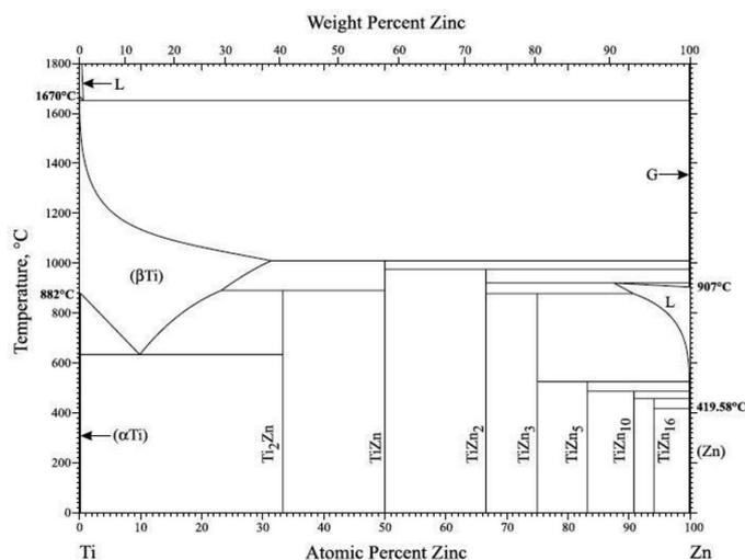
Fig. 1. Zn-Ti phase diagram, Okamoto 2008 [8]
