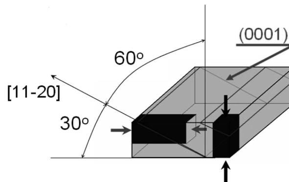
Fig. 2. Primary single crystal and cut off method of samples for the compression test
