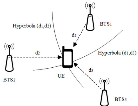
Fig. 4. E-OTD positioning method
