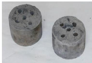
Fig. 7. Ready briquettes containing post-reclamation dust bonded with cement binder
