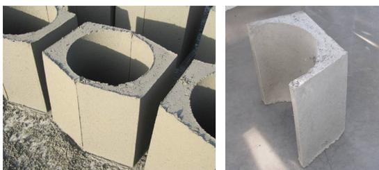
Fig.6. Ready concrete products (drain pan) made of concrete with the reclaimed sand before and after aging
