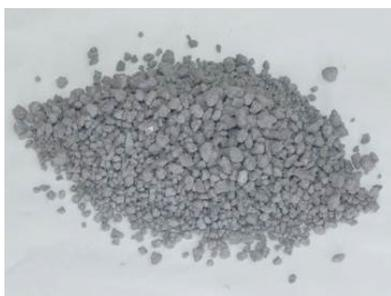
Fig.8. A sample of the granulated post-reclamation dust
