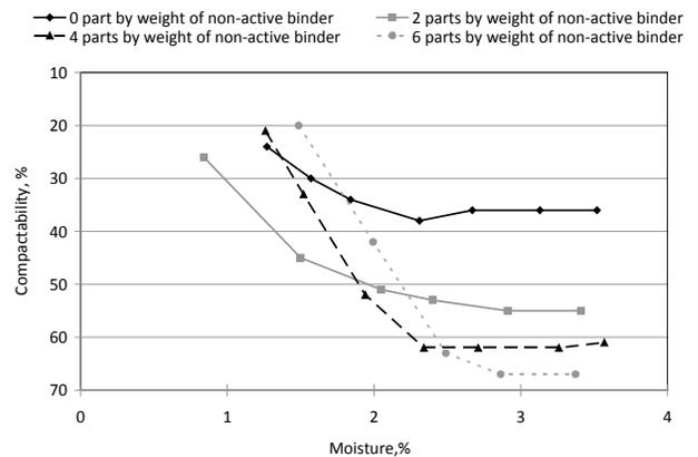
Fig. 3. The influence of water content on compactability, for the moulding sands with different active bentonite content
