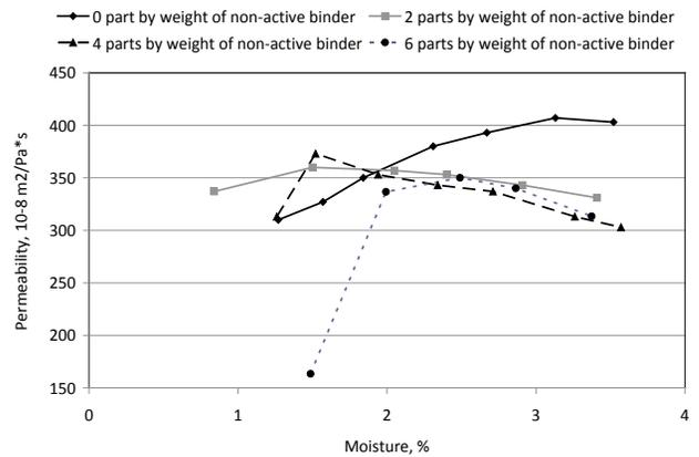
Fig. 2. The influence of water content on permeability for the moulding sands with different active bentonite content
