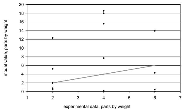
Fig. 7. Comparison of the distribution of data generated by the network and the experimental data (test data), input data: compressive strength, compactability, permeability
