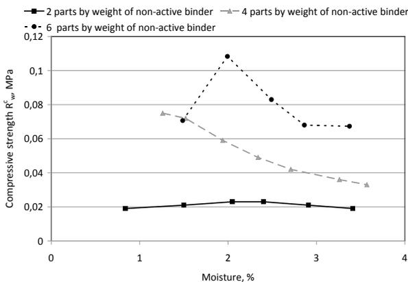
Fig. 1. The influence of water content on compressive strength  $R_c^w$ , for the moulding sands with different active bentonite content
