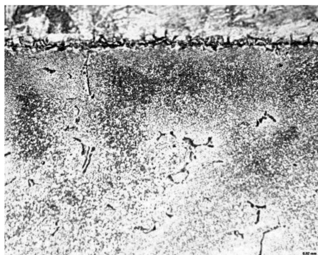
Fig. 5. Microstructure of the stainless steel (X2CrNi 18-9) joint brazed with BAG-19 alloy. Upper part – stainless steel, lower part – braze
