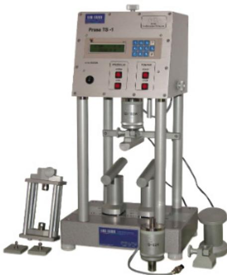
Fig. 7. The stand for bending tests [14]
