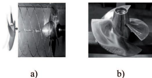
Fig. 1. Screw propeller damage caused by cavitation process
