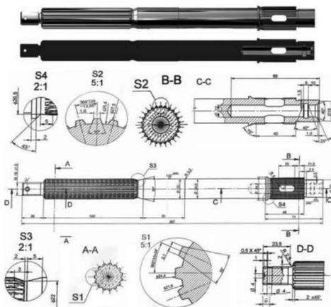
Fig. 2. Driving shaft  $\varnothing 335$  of the motor boat screw propeller (Type OP-1960-00-04/1)
