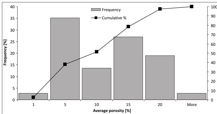
Fig. 7. Average porosity distribution for analyzed oil fields
