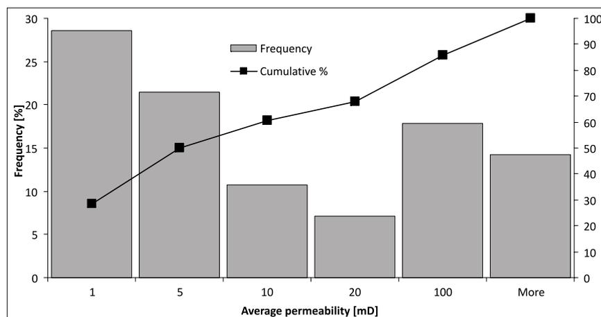
Fig. 6. Average permeability distribution for analyzed oil fields
