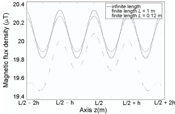
Fig. 2.  $B_\phi$  component versus  $z$  ( $h = 2$  cm)
