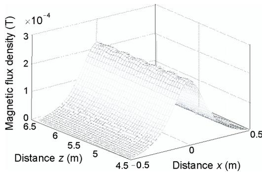
Fig. 4. Distribution of the magnetic field density in the  $xz$ -plane at radial distance 5 cm from center of the 3-phase cable
