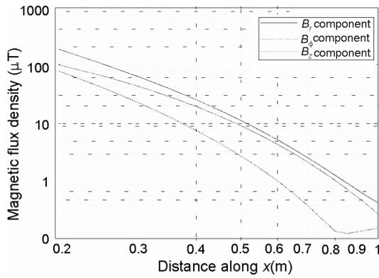
Fig. 3. Components of the magnetic field density as function of radial distance from axis of the 3-phase cable
