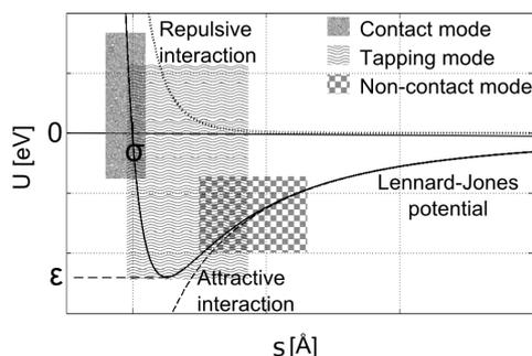
Fig. 3. Sketch of a typical tip-sample potential
