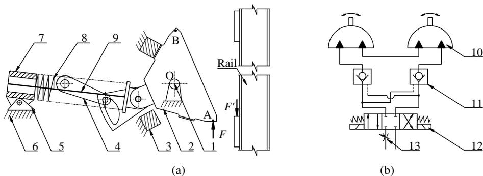
Fig. 5. The new rail clamping device: a) the structure diagram of the clamping device; b) a hydraulic circuit for controlling rotary actuators. 1. horizontal shaft, 2. anchor, 3. bearer, 4. shake bar, 5. lid, 6. clamp housing, 7. shaft button, 8. spring, 9. inclined shaft, 10. hydraulic rotary actuator, 11. pilot-operated check valve, 12. directional valve, 13. variable throttle valve
