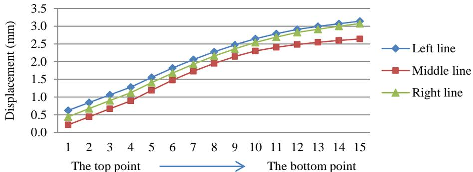
Fig. 10. Investigating the horizontal displacement of the shell by the height
