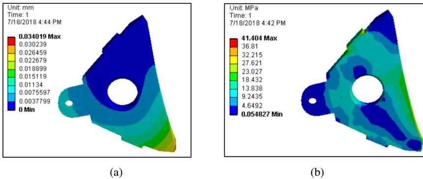
Fig. 8. The values of stress and displacement of the anchor
