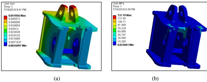
Fig. 9. The values of stress and displacement of the clamp housing
