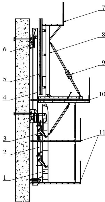
Fig. 1. Structure diagram of a self-climbing formwork. 1. lifting frame, 2. hydraulic system, 3. rail climbing device, 4. rail, 5. formwork shell, 6. climbing shoes, 7. concreting platform, 8. main frame, 9. cross brace, 10. main platform, 11. under platform
