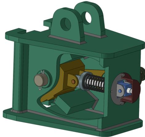
Fig. 6. 3D simulation of the rail clamping device
