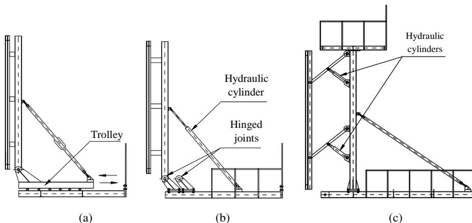
Fig. 2. Method for opening and closing the formwork shell by: a) trolleys, b) hydraulic cylinders and articulate joints, c) hydraulic cylinders and arms arranged parallelogram style
