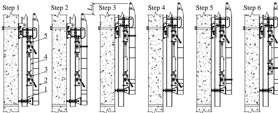
Fig. 4. A lifting cycle of the lifting frame. 1. rail, 2. lifting frame, 3. under rail clamping device, 4. hydraulic cylinder, 5. upper rail clamping device
