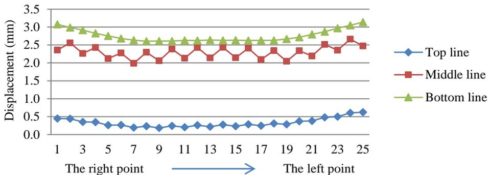
Fig. 11. Investigating the horizontal displacement of the shell by the length
