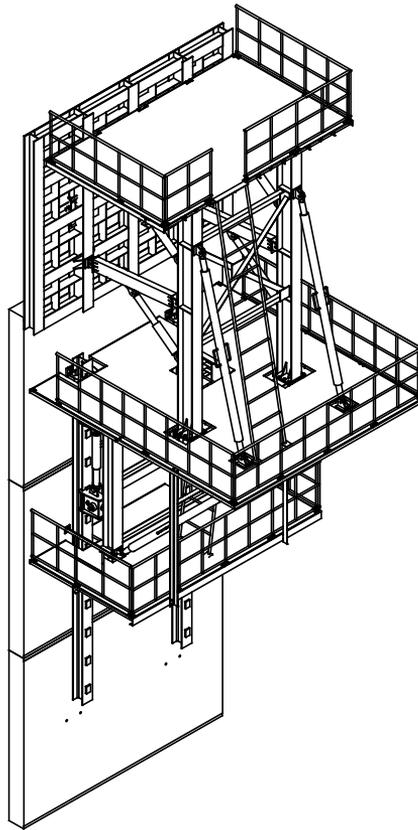
Fig. 7. The hydraulic self-climbing formwork with the shell's working size of  $4\text{ m} \times 3\text{ m}$
