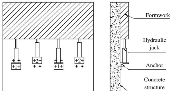
Fig. 3. Principle of the lifting process of formworks by hydraulic jacks with a parity type
