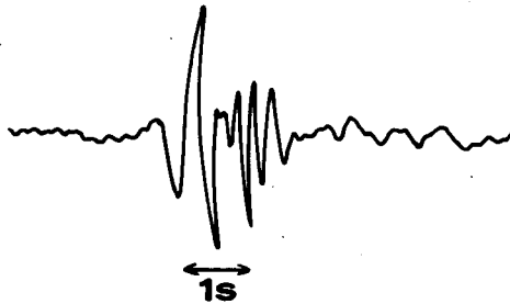
Fig. 6. Seismogram of an impulse generated by an iceberg seated on the sea bottom
