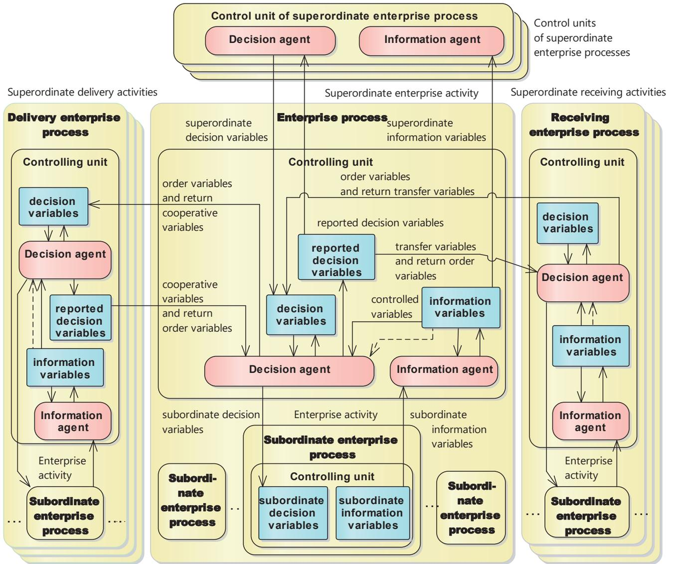
Fig. 5. Information flow between functional agents of enterprise process
