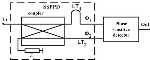
Fig. 8. A block diagram of a “sine” type frequency detector.
