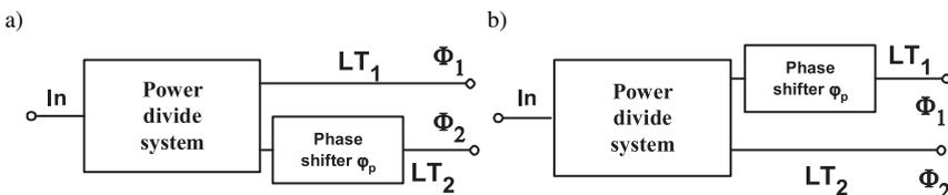
Fig. 6. Modifications of the system of developing a proportional phase difference.
