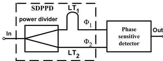
Fig. 4. A block diagram of a “cosine” type SFD.
