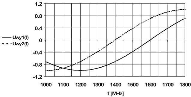
Fig. 10. Characteristics of output voltages for a “sine” type SFD without a phase shifter and with a phase shifter for  $n = 1$  (solid line – a curve of output voltage for the frequency detector without any interference in the SDPPD structure, dashed line – a curve of output voltage for the detector after introducing a phase shifter).
