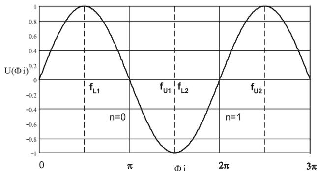
Fig. 9. Ranges of an unambiguous reading of frequencies for a “sine” type detector of frequency.
