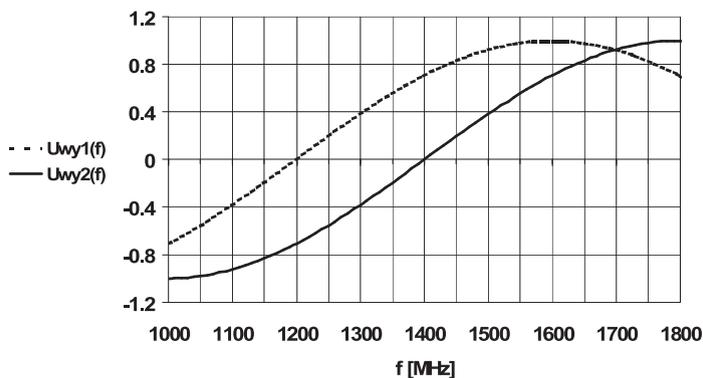
Fig. 7. Characteristics of input voltage for a “cosine” type SFD operating in a range of 1–1.8 GHz without a phase shifter and with a phase shifter with a shift of 45 degrees for  $n = 1$  (solid line – a curve of SFD output voltage with a phase shifter, dashed line – a curve of output voltage without a phase shifter –).
