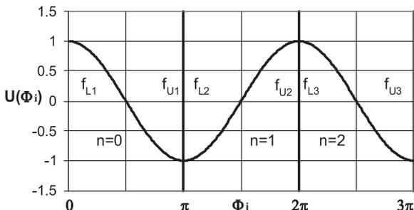
Fig. 5. Ranges of unambiguous reading of frequency by a “cosine” type frequency detector.
