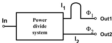
Fig. 2. A block diagram of System of Developing a Proportional Phase Difference.
