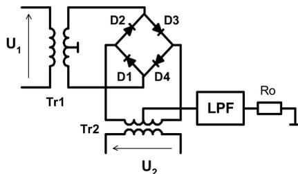
Fig. 3. A schematic diagram of a phase-sensitive detector with a diode ring.
