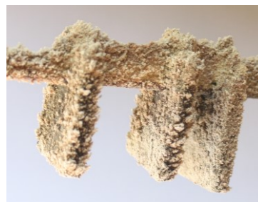
Fig. 1. A view of specimens after a 30-day test. Note the deposit of solid combustion products
