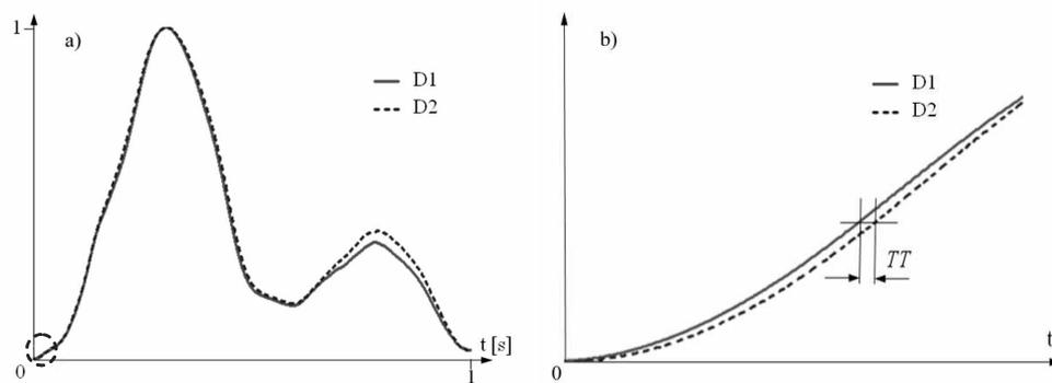
Fig. 3. a) Normalized pulse waves (the internal diameter D1 and D2 of the pipe) measured at two points of the model of the artery, b) zoom of region  $z$  marked by dashed circle in a), where the transit time of the pulse wave  $TT$  was determined.
