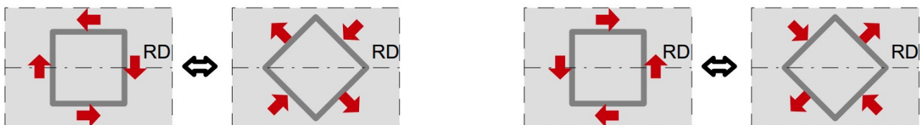
Fig. 2. Lack of SDE when shearing along the rolling direction (RD) and the transverse one
