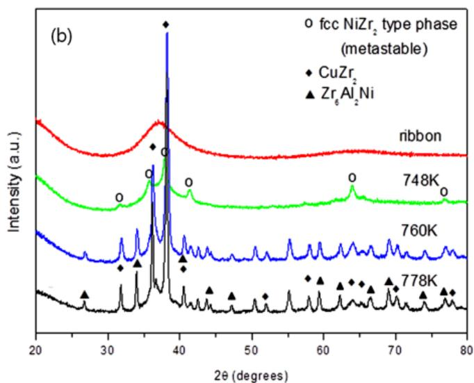
Fig. 3. (a) DSC curves and (b) XRD trace of the  $\text{Zr}_{62}\text{Al}_8\text{Ni}_{13}\text{Cu}_{17}$  metallic glass annealed at different temperatures
