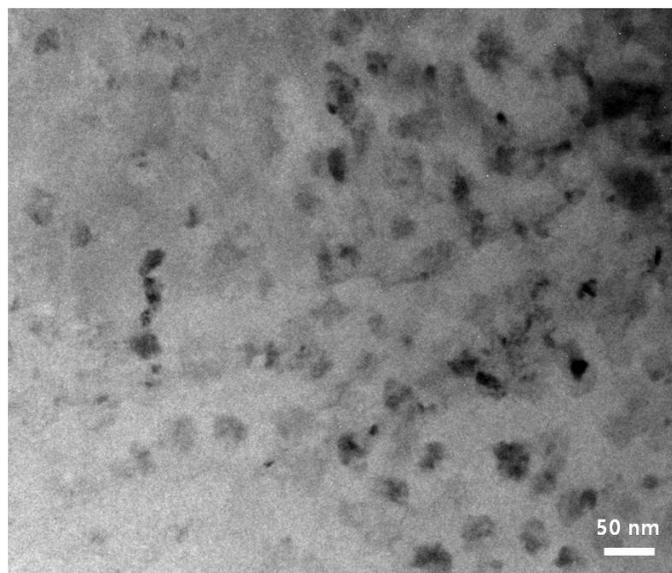
Fig. 6. Typical bright field TEM image obtained from  $Zr_{62}Al_8Ni_{13}Cu_{17}$  ribbon specimen annealed for 60 s at 778 K
