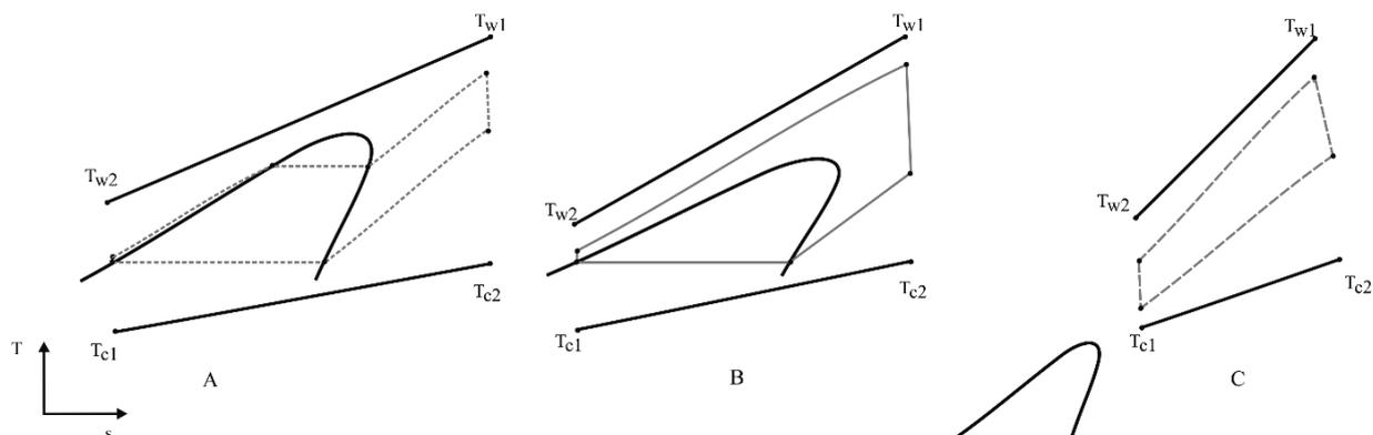
Fig. 1. Illustrative representation of cycles: A – vapour, subcritical, B – vapour, supercritical, C – single-phase vapour (gas) implemented at the same initial temperatures of the upper ( $T_{w1}$ ) and the lower heat source ( $T_{c1}$ )
