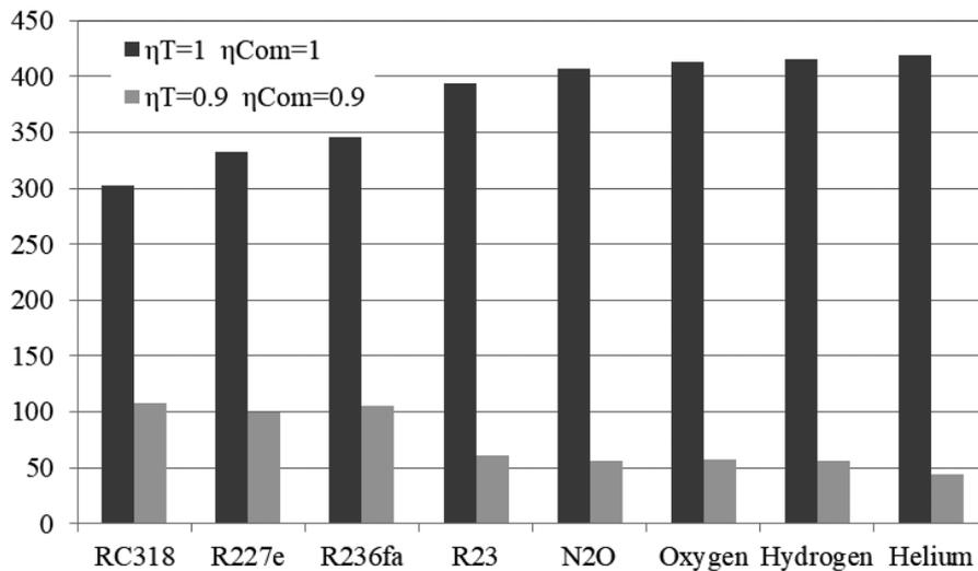
Fig. 3. Comparison of the Brayton cycle power values with different working fluids, for optimum pressure ratios, assuming different turbine and compressor internal efficiency
