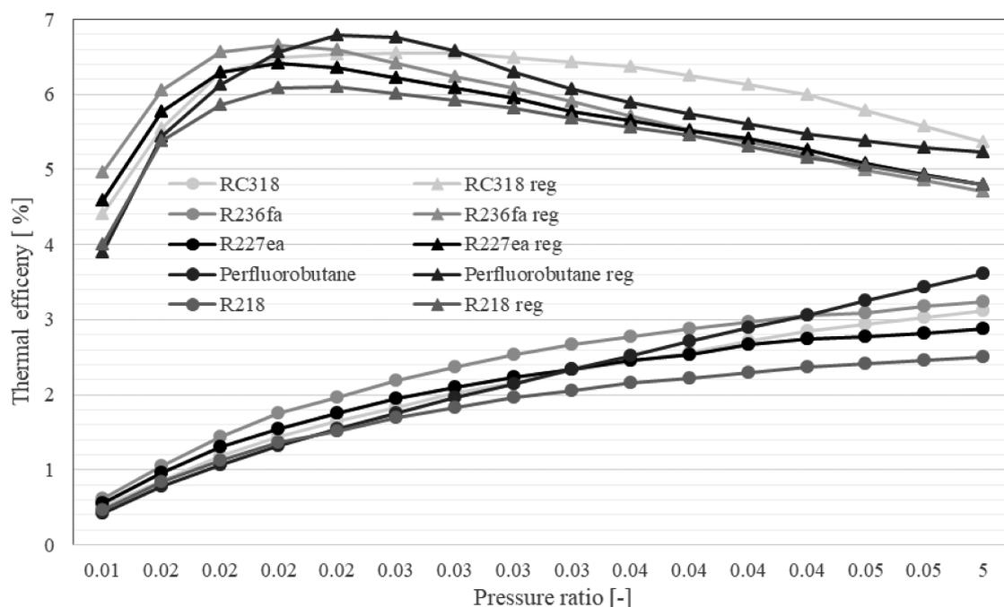
Fig. 5. Efficiency of the organic Brayton cycle with and without the use of internal heat regeneration, supplied from a source of temperature  $160^{\circ}\text{C}$  ( $\eta_T = 0.9$ ,  $\eta_{Com} = 0.9$ )
