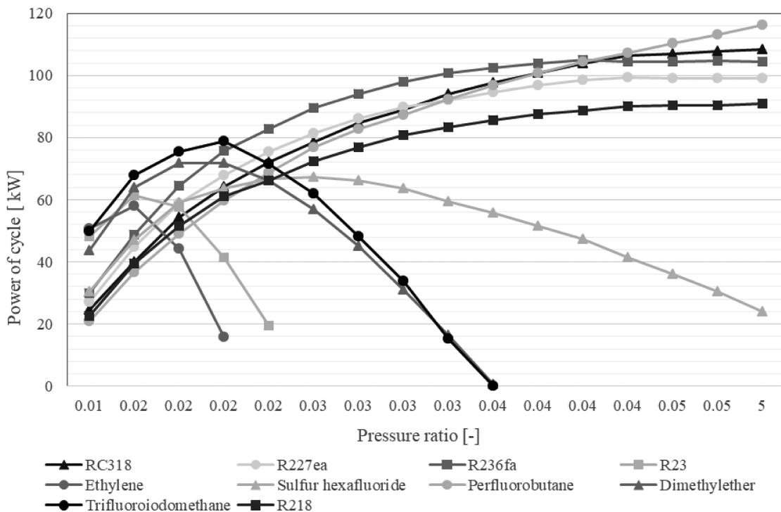
Fig. 4. The Brayton cycle power with various organic working fluids supplied from the source with a temperature of 160°C, assuming that internal efficiency of the turbine and compressor is  $\eta_T = 0.9$ ,  $\eta_{Com} = 0.9$ , respectively
