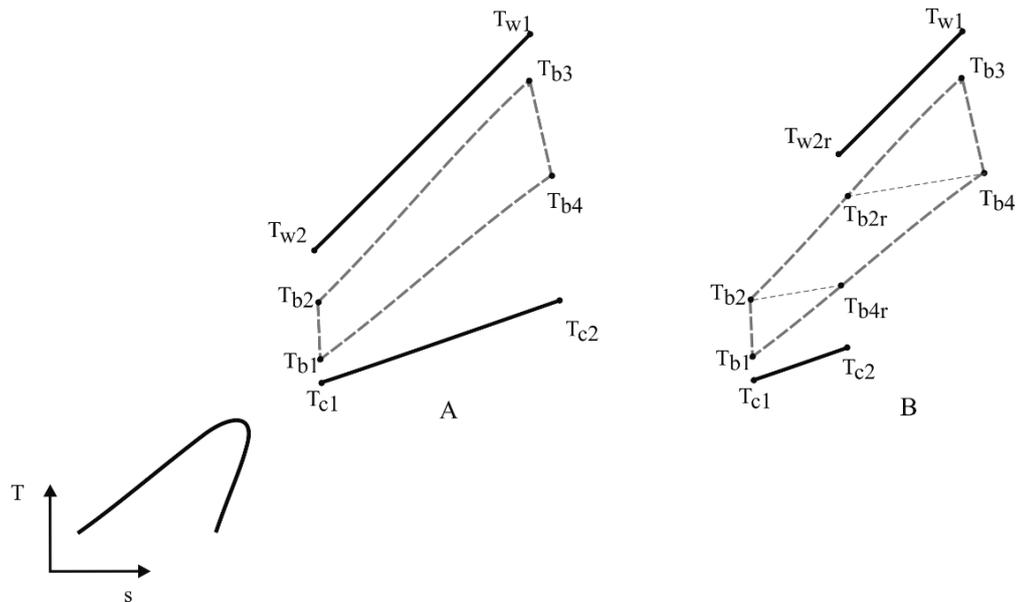
Fig. 2. Thermodynamic processes of the Brayton cycle A) without heat regeneration; B) with internal heat regeneration
